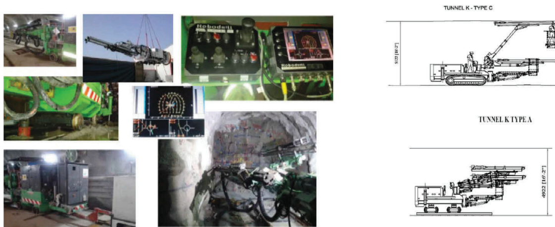
Figure 12. Jumbos switchable from wheels to rail undercarriage.
