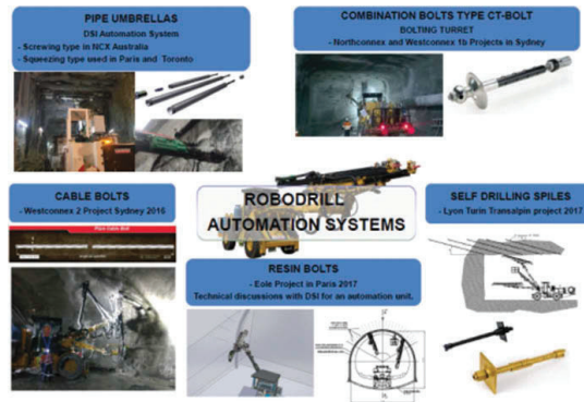
Figure 1. Example of different bolt types which can be installed automatically by the drilling system.
