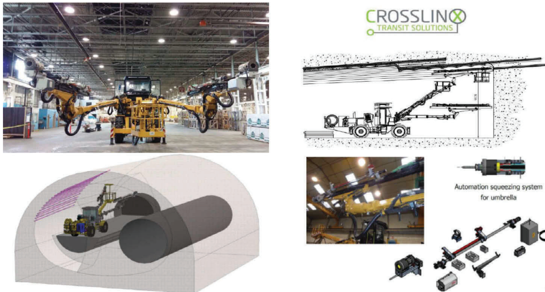
Figure 9. Jumbos provided with drifters and automatic squeezing system for DSI pipe umbrella.
