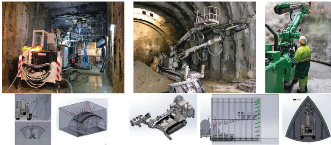
Figure 16. Customized jumbos for special application in Gran Paris.
