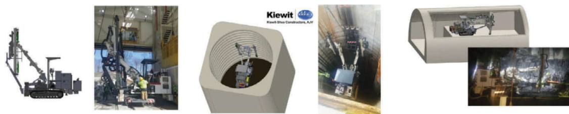
Figure 5. Shaft jumbo able to perform vertical and horizontal drilling operations.
