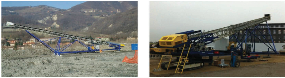
Figure 7. Special belt conveyor to spread out the muck.
