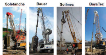
Figure 6. Some of the main brand of foundations rig with grab.
